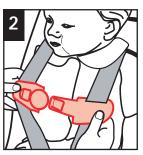
Press on harness retainer release button and pull apart.
